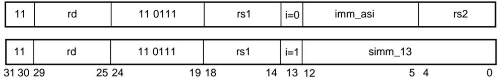
**Figure 13-35** Format (3) STDFA:**Table 13-29** Block Load and Store Instruction Syntax
